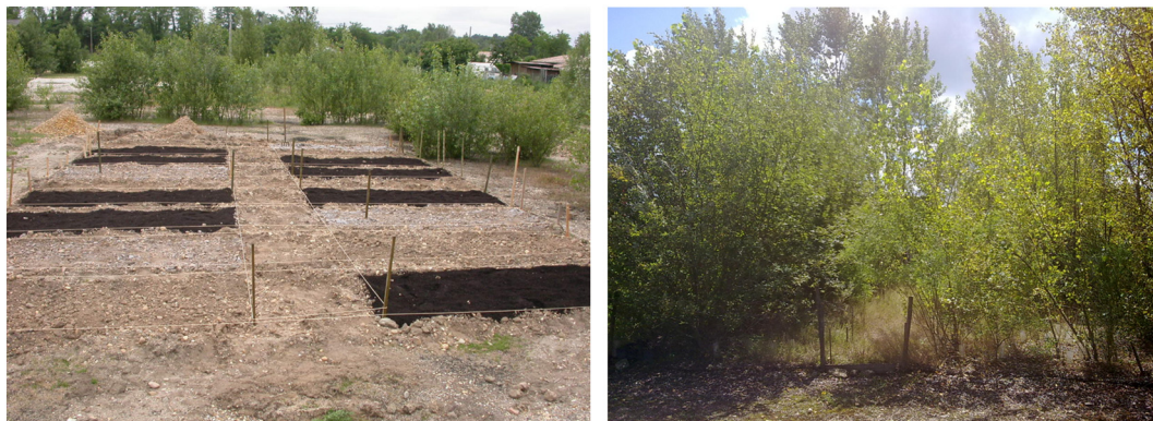
Fig. 5. Field trial with compost amendment at a former wood preservation site, St-Médard d'Eyrans, France. Short rotation coppice (black poplar and willows) in year 6 after the compost incorporation into the soil and transplantation of mycorrhizal trees. Soil is remediated and prepared to multiple uses, see also table in the supplemental material (Photos: M. Mench).
